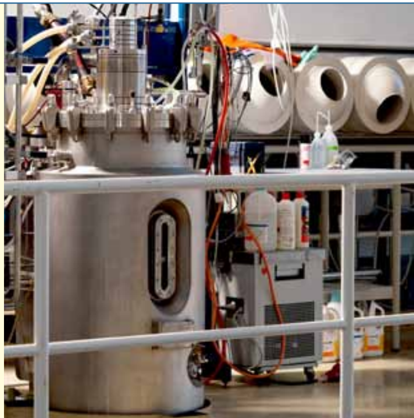
One of the 300-l fermenters in the laboratory of the Institute of Biochemical Engineering.
