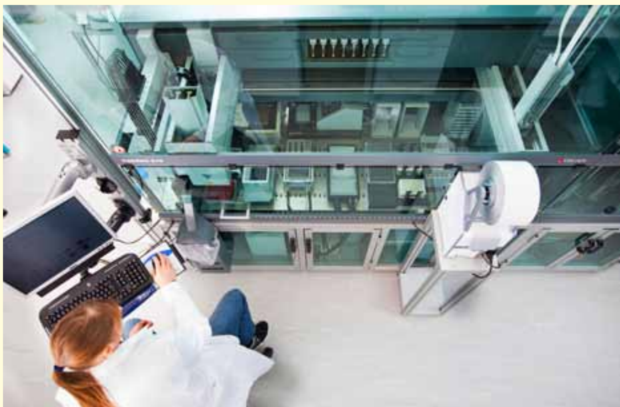
Laboratory automation system at the Center for Biological Systems Analysis (University of Freiburg). This robotic platform is used for high-throughput molecular biology screening and combinatorial experiments.
