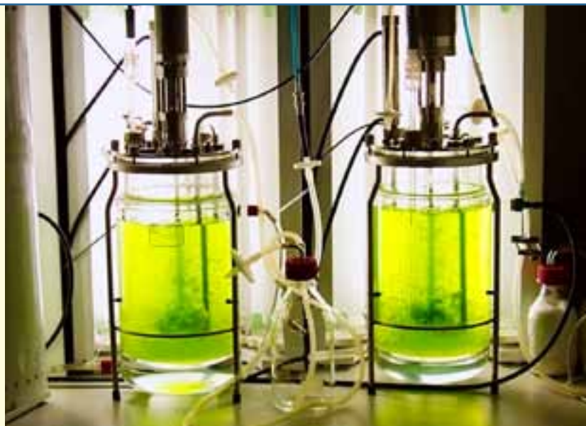
Photobioreactors with moss cultures for the production of complex biopharmaceuticals (molecular farming).
