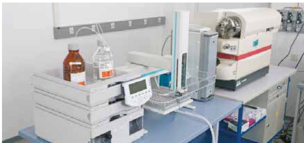
HPLC with autosampler and -MS/MS Massspectrograph (Agilent/Applied Biosystems)
